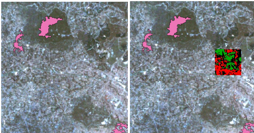
Figure 11: example of image with selected ROIs (left) and preview of classification (right)
